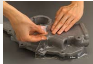
PhotoStress coating applied to a structure of complex shape
