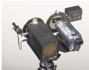
LF/Z-2 Reflection Polariscope— tripod-mounted or handheld
